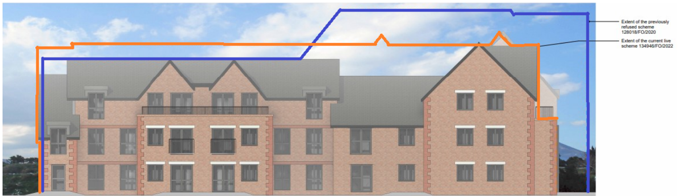
Proposed East Elevation of revised scheme – Blue line indicates building line of previously refused scheme, the orange line shows the building line of the scheme as originally submitted
