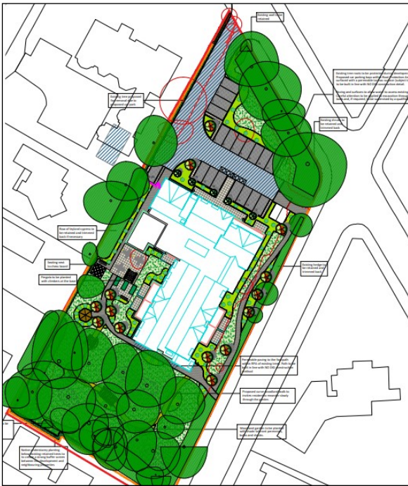
Proposed site layout shown the outline of the proposed building, tree cover, parking and the relationship with neighbouring properties
