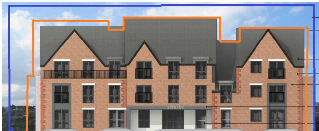
Proposed North Elevation of revised scheme - Blue line indicates building line of previously refused scheme, the orange line shows the building line of the scheme as originally submitted
